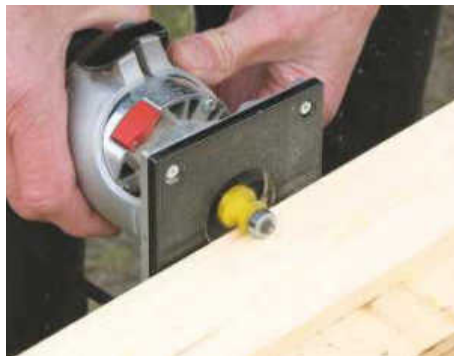
STEP 12. The upper and lower aprons all feature decorative beading. Rout this carefully with a bearing-guided cutter
